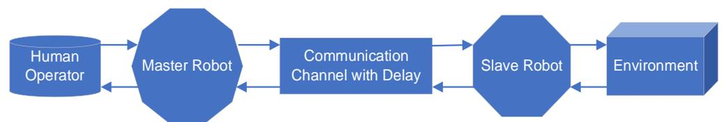
**Figure 1.** The control structure of the bilateral teleoperation robot system.
