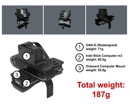
**Figure 5.** The 3D-printed mount to carry the OAK-D smart camera (with the new back case) and the Intel Compute Stick onboard the drone.
