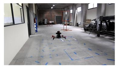
**Figure 11.** Indoor environment for our experiments where the drone had to fly through gates. All processing was performed on board using an OAK-D smart camera and an Intel Stick Compute processor.
