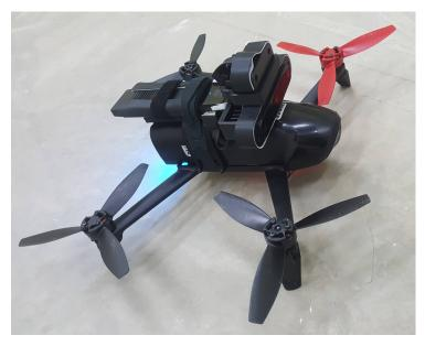
**Figure 3.** First mount design enabling the Bebop 2.0 Power Edition to carry the Intel Compute Stick and the OAK-D smart camera with its original case. In this design, the total weight was 283 g, 117 g for the OAK-D sensor, plus 166 g for the onboard computer and the mount. This exceeds the maximum payload set by us (200 g) by 83 g, which resulted in unstable flights.
