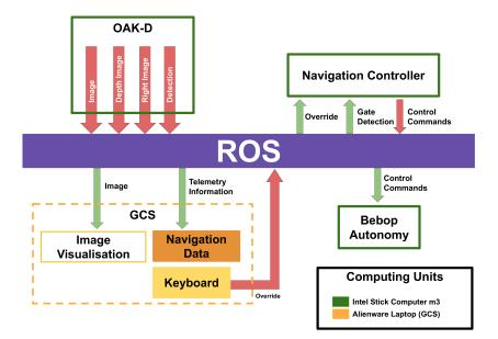
**Figure 9.** Communication system based on the robotic operating system. Nodes running on the Intel Stick (full onboard processing) are marked in green. Nodes running on the ground control station (GCS) are marked in orange. The GCS is only used for visualisation of imagery and telemetry transmitted by the system running onboard the drone.
