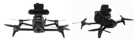
**Figure 6.** Front and side views of the Bebop 2.0 Power Edition carrying the OAK-D and the Intel Compute Stick.
