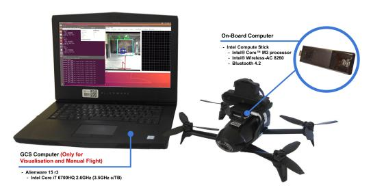
Figure 10. GCS and the Bebop 2.0 PWE with the Intel Stick and the OAK-D camera on board.
