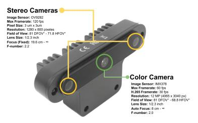
**Figure 1.** OAK-D is a camera capable of running neural networks simultaneously while providing depth from two stereo cameras and colour information from a single 4K camera in the centre. The camera's weight is 117 g, and its dimensions are 110 mm in width, 54.5 mm in height, and 33 mm in length.
