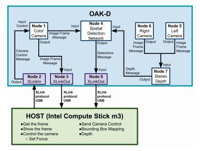
**Figure 2.** General diagram of the internal configuration of the OAK-D camera to obtain colour camera images, an object of interest, and their spatial position with respect to the camera.
