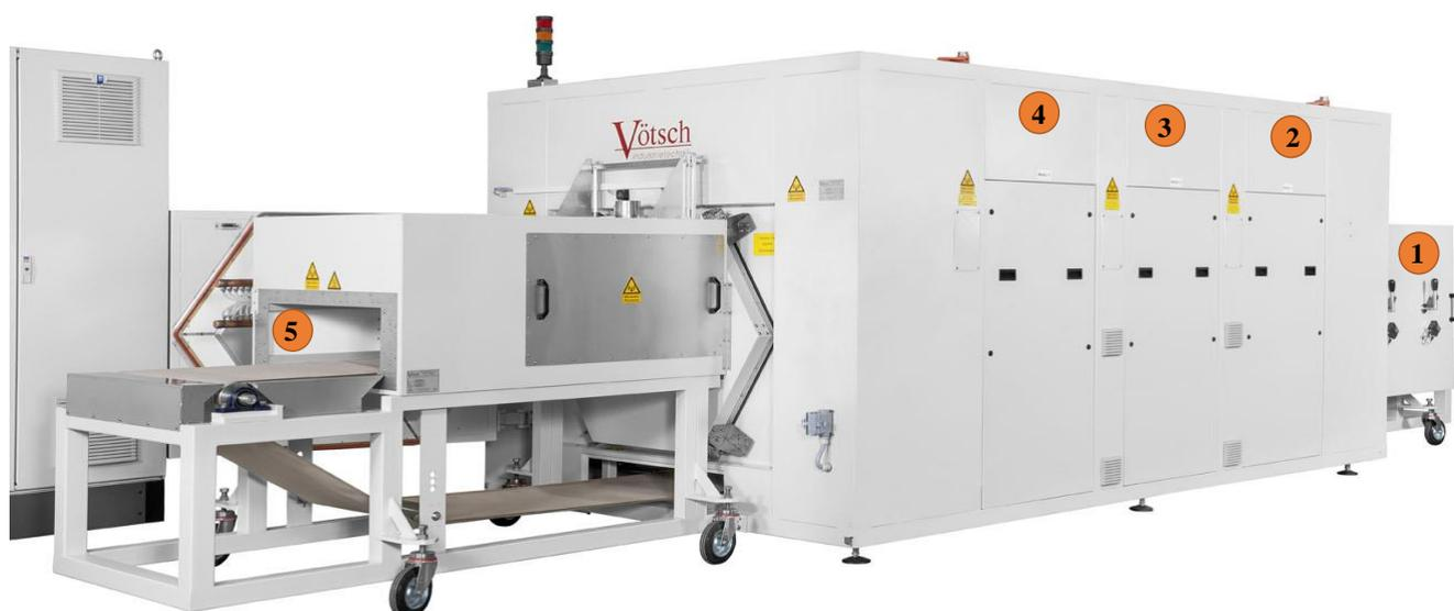
**Figure 1.** A side view of the HEPHAISTOS microwave oven system. Main modules of the oven are represented by number tags 1, 2, 3, 4, 5. Tag 1 and Tag 5 represent the entrance of the wet foam and exit doors for the dry foam on the conveyor belt, respectively. Tags 2, 3, 4 indicate the three modular heating systems which are built into the hexagonal cavity with high power microwave heating sources and control system block.
