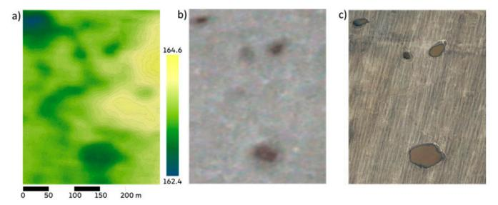
**Figure 2.** Sources of spatial data. (a) High-resolution DEM obtained photogrammetrically with colors indicating heights. (b) Planet Labs' digital images of terrain in the visible spectrum with 3 m resolution. (c) High-resolution digital image obtained using the UAV in the visible spectral range.
