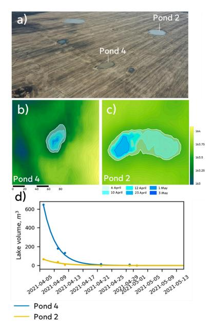
**Figure 4.** Temporal dynamics of selected ponds in the depressions. (a) Positions of Ponds 4 and 2 in a UAV photo image. (b,c) Groundwater levels in basins of the ponds on indicated dates based on the classification of images (highlighted in color by day). (d) Water volumes in the basins of ponds 4 and 2 on indicated dates (points) and negative exponential fits derived by Equation (8) (lines). Pond numbering as in Figure 1 and Table 2.
