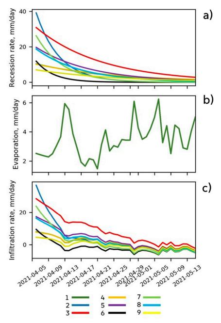
**Figure 5.** Rate of recession of the indicated ponds' water levels (a), daily evaporation rate (b) and infiltration rates of the ponds estimated from the mass balance (bottom panel) expressed in mm of the water layer (c). The numbering of the ponds in the color legend follows Figure 1 and Table 2.
