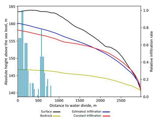
**Figure 7.** Cross-section of the catena with water table depth (WTD, blue and red lines) adjusted to correspond to soil group [22]. The yellow and black lines indicate the position of the bedrock and DEM profile, respectively. The blue and red lines respectively indicate WTD obtained with infiltration along the transects estimated from the depressions' positions and specific infiltration rates (as indicated by the blue bars and right y axis) and constant infiltration along the transect.
