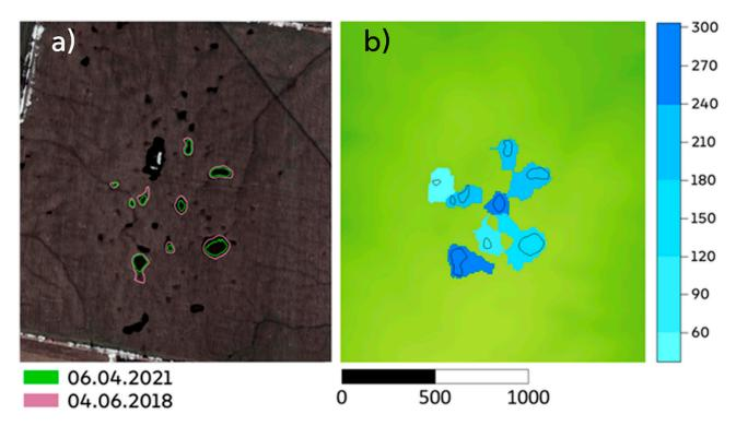
**Figure 6.** (a) Boundaries of the maximum potential filling of closed depressions (up to their overflow heights) shown in white in a Planet Labs image from 4 April 2018, with color shading and magenta contours, and the maximum pond boundaries in 2021 from 6 April 2021 (green contours). In 2018, the investigated closed depressions were overflowing. (b) Shades of blue indicating the layers of water (in mm) that must enter the depressions from their catchment areas to completely fill them.
