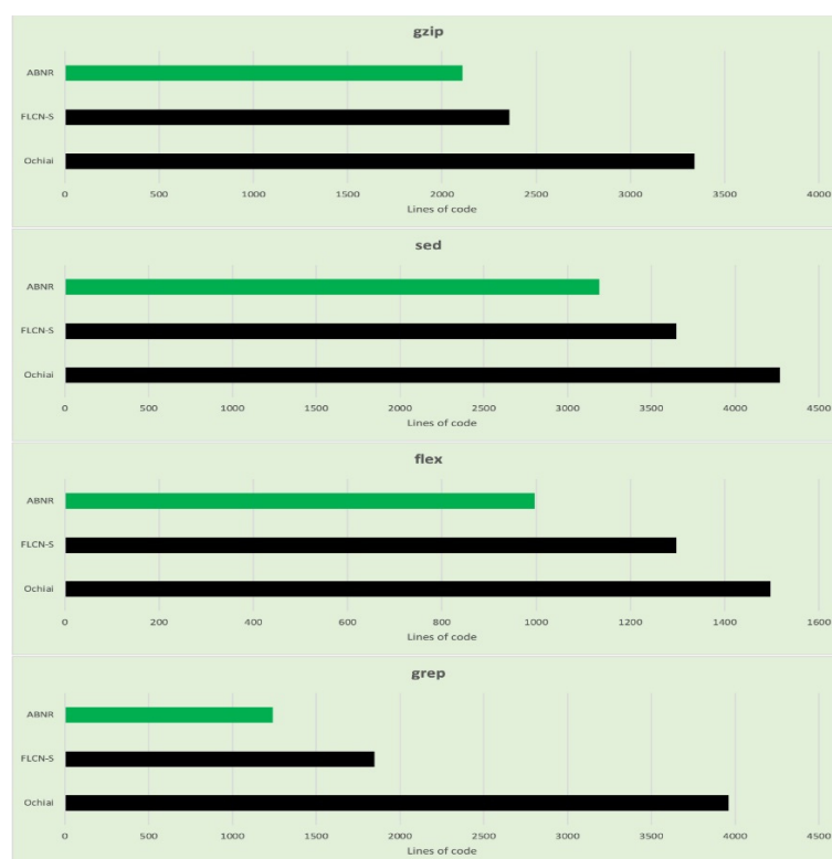
Figure 6. Graphs representing the number lines of code evaluated for fault localization for each category in the Unix utility program.
