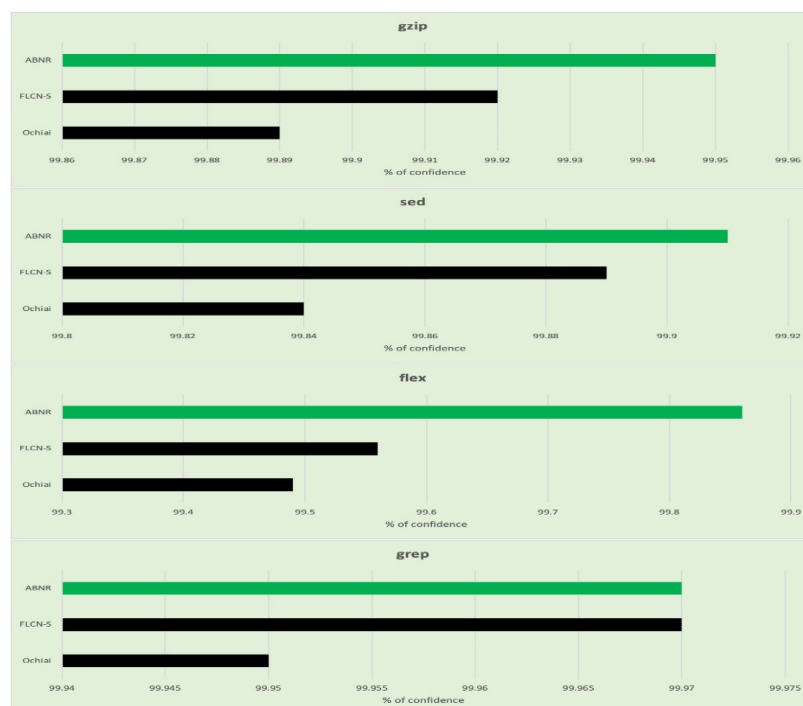
Figure 8. Graphs representing the confidence level of fault localized for each category in Unix utility applications.
