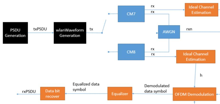
Figure 2. Block diagram model for reliability analysis.
