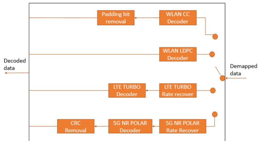
Figure 6. Proposed decoding structure.
