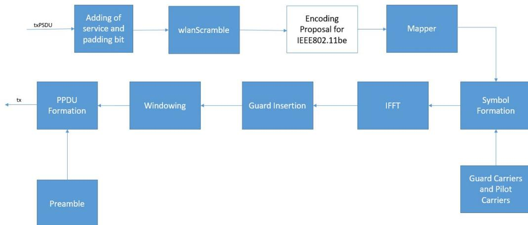
Figure 3. wlanWaveform structure.
