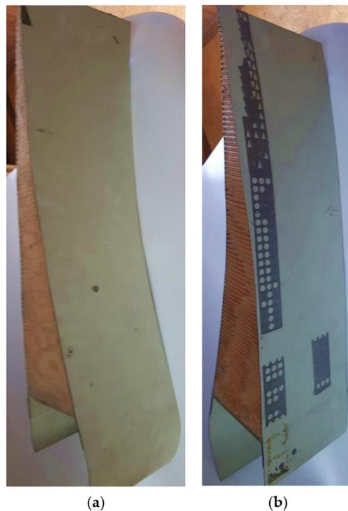
**Figure 13.** NDE test pieces (landing flap transversal portion, containing mainly air) of (a) Boeing-777 plane wings, fabricated for the maker (b) with internal artificial flaws located in unknown locations.
