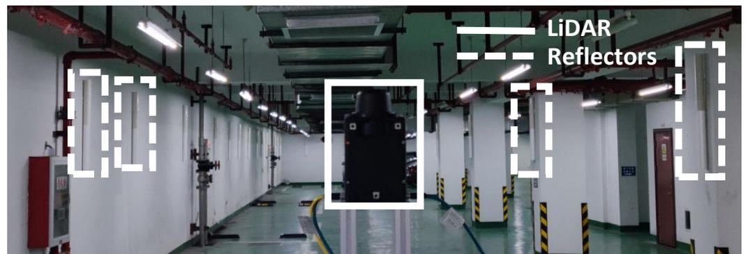
**Figure 1.** Hardware required for the reflector positioning system. The black device indicated by the solid line is a 2D LiDAR. The white pipes indicated by dotted lines are reflectors.
