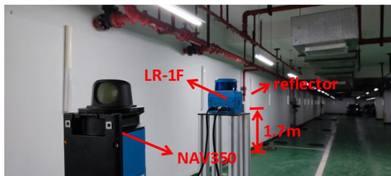
**Figure 15.** The platform and environment of the experiment. The height of LR-1F was set to 2 m and NAV350 was slightly lower than that of LR-1F. The experimental environment was an L-shaped underground garage about 50 m long and 5 m wide. The reflectors were randomly suspended on the wall with a height of 1.7 m.
