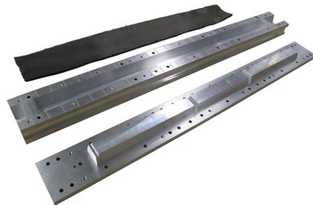
**Figure 4.** Casket molding (from the top): Carbon fiber sheets, heatable female mold and male mold.
