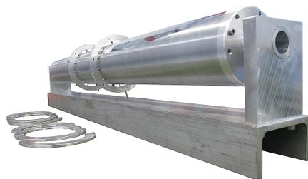
**Figure 5.** Mandrel for the fabrication of the inner carbon fiber cylinder.
