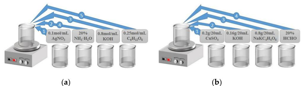
Figure 5. (a) Preparation process of reagent required for silver mirror reaction; (b) Preparation process of reagent required for bronze mirror reaction.
