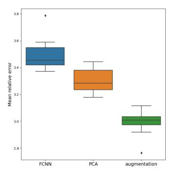
**Figure 5.** Distribution of mean relative percentage errors for 3 models: baseline model, model trained on PCA features and model trained on augmented data.
