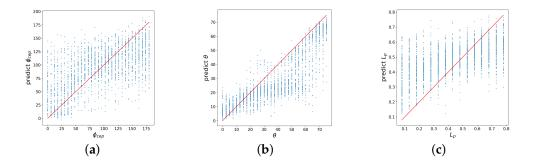
**Figure 7.** Correlation of the exact and predicted values of laser–plasma interaction parameters, reconstructed by a baseline fully connected NN trained on clean data and tested on noisy data: (a) carrier envelope phase, (b) incidence angle, (c) pre-plasma length.
