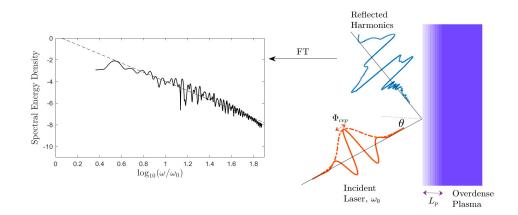
**Figure 1.** A schematic diagram showing the simulated scenario. A laser pulse angularly incident on a solid plasma target with a pre-plasma length. The reflected spectrum contains harmonics of the laser's initial frequency, and the intensity of these harmonics decays with increasing harmonic order.
