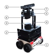
**Figure 2.** An overview of the mechanical design of ROBOGait. The figure shows: (1) the mobile robotic base, (2) on-board computer (Intel NUC), (3) Slamtec LIDAR A2 sensor, (4) adjustable aluminum brackets, (5) servoing system mechanism, (6) servomotor (Hitec HS-755HB), (7) damping device, and (8) Orbbec Astra RGBD camera.
