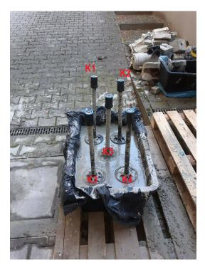
Figure 14. Laboratory model of bolted roof.
