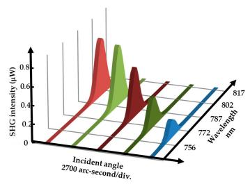
Figure 7. Characteristic of SHW spectra in different incident angles using LiNbO<sub>3</sub> crystal.
