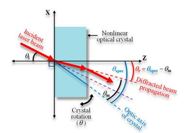
**Figure 4.** Schematic of refraction effect due to crystal diffraction; the change in direction of an incident laser beam through a nonlinear optical crystal.
