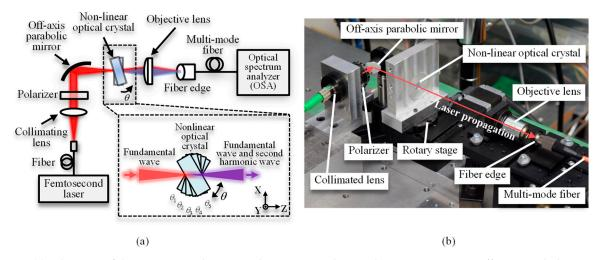
**Figure 5.** (a) Schematic of the experimental setup to observe FW and SHG phenomena using an off-axis parabolic mirror for beam focusing; (b) a photograph of the experimental setup.
