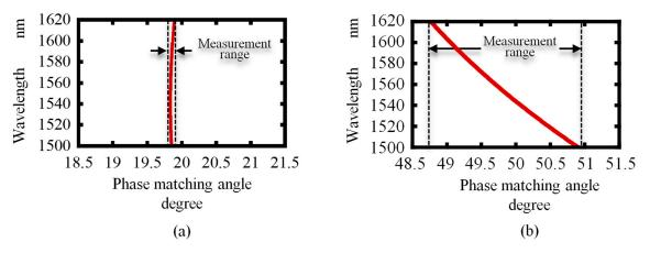
Figure 3. Wavelength-dependent phase-matching angle: (a) BBO; (b) MgO: LiNbO<sub>3</sub>.
