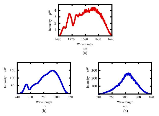
**Figure 6.** (a) FW spectrum before conversion; (b) second harmonic wave (SHW) spectrum focusing by a parabolic mirror; (c) SHW spectrum focusing by a lens.
