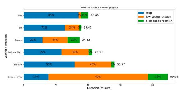
Figure 4. Washing time configurations for different washing programs.
