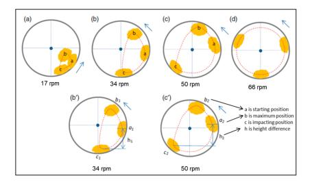
**Figure 9.** Fabric movement in the washing drum, (a) 17, (b) 34, (c) 50, and (d) 66 rpm [38]. (Reproduced with permission).
