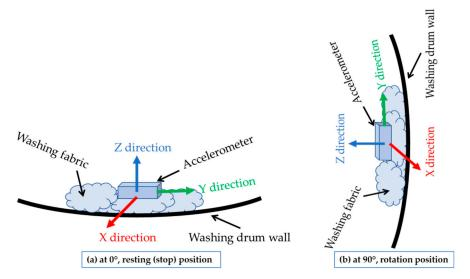
**Figure 6.** Coordinate system (X, Y, and Z) of the accelerometer fixed to the plain fabric that was moving during the washing cycle (**a**) at the  $0^{\circ}$  position and (**b**) at the  $90^{\circ}$  position.
