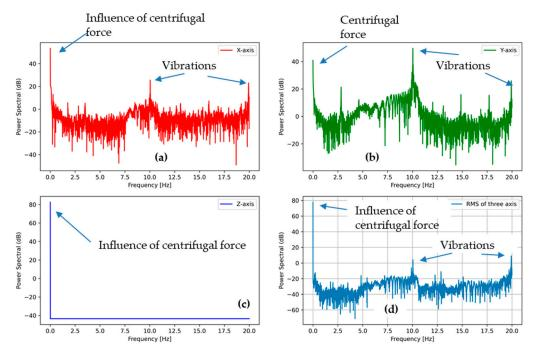
**Figure 14.** PSD of the accelerometer outputs from the tumble phase (600 RPM) (after removing initial acceleration phase) (a) in the X direction, (b) in the Y direction, and (c) in the Z direction, (d) the sum of all the accelerations.
