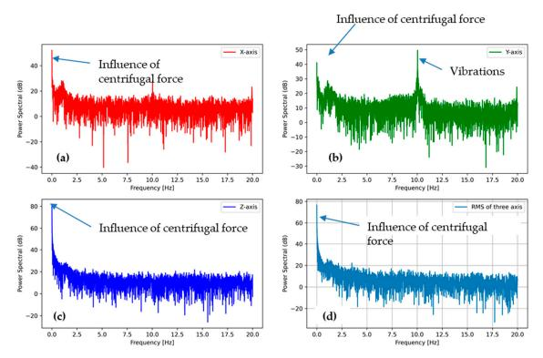
**Figure 12.** PSD of the accelerometer outputs from tumble phase (600 RPM) (**a**) in the X direction, (**b**) in the Y direction, and (**c**) in the Z direction, (**d**) the sum of all the accelerations.
