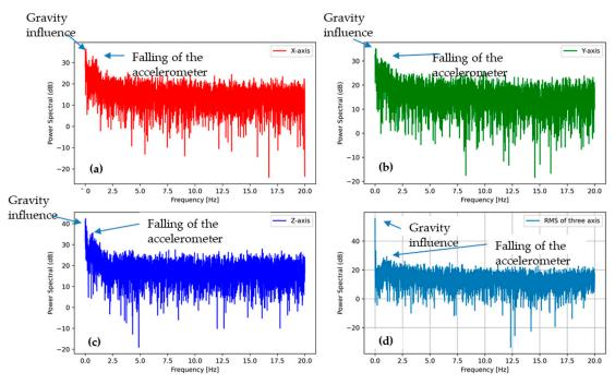
**Figure 10.** Power spectral density (PSD) of the accelerometer outputs of washing phase (low-speed rotation action) (a) in the X direction, (b) the Y direction, and (c) the Z direction, as well as (d) the sum of all the accelerations.
