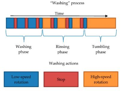
Figure 3. Configuration of washing phases and actions.
