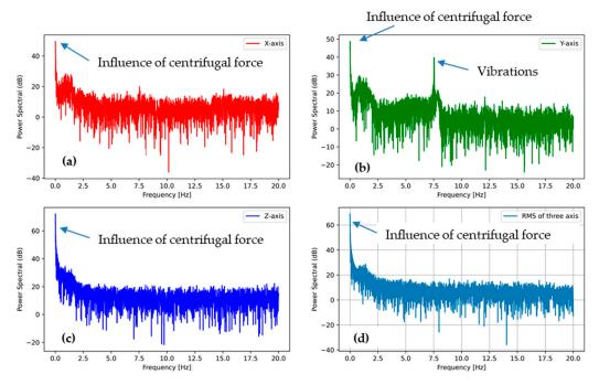
**Figure 11.** PSD of the accelerometer outputs from tumble phase (high-speed rotation 400 RPM) (**a**) in the X direction, (**b**) in the Y direction, and (**c**) in the Z direction, (**d**) the sum of all the accelerations.
