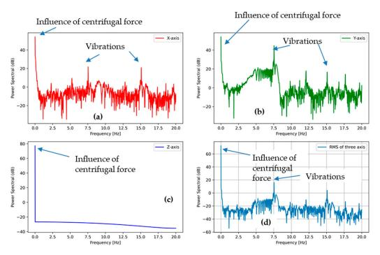
**Figure 13.** PSD of the accelerometer outputs from the tumble phase (400 RPM) (after removing initial acceleration phase) (a) in the X direction, (b) in the Y direction, and (c) in the Z direction, (d) the sum of all the accelerations.
