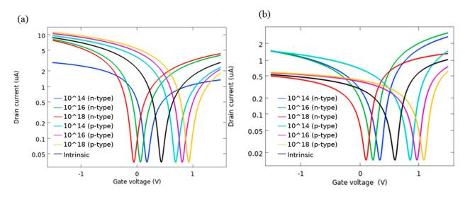
Figure 11. I-V characteristics as a function of doping type and concentration for (a) AlP-GFET, (b) Pd- GFET.
