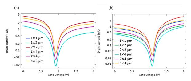
**Figure 10.** I-V characteristics as a function of channel dimension (W × L), for (**a**) AlP-GFET (**b**) Pd-GFET. The I<sub>d</sub> of the devices with equal  $\frac{W}{T}$  ratios are overlapped.
