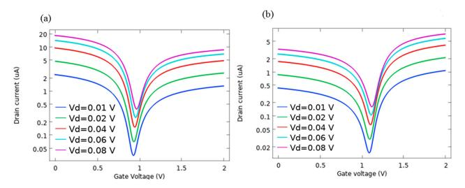
**Figure 9.** I-V characteristics as a function of applied  $V_d$  for (**a**) Al-P doped GFET (**b**), Pd-decorated GFET. According to the graphs,  $V_n$  of the devices remains constant as  $V_d$  varies.
