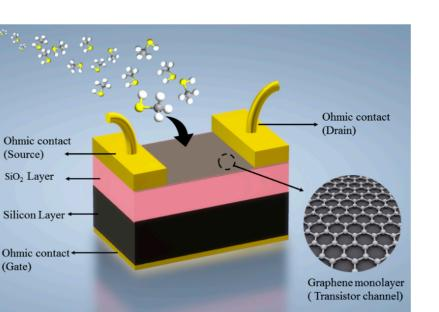
**Figure 1.** The proposed graphene field effect transistor (GFET) model. The back-gate structure enables binding of the biomarker to the channel surface.
