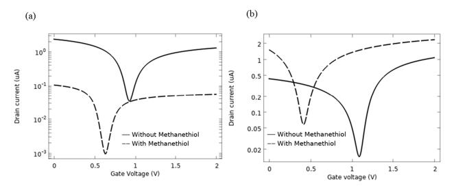
Figure 13. I-V characteristics before and after adsorption of methanethiol for (a) AIP-GFET, (b) Pd-GFET.
