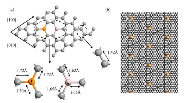
**Figure 2.** Ground-state optimal structure of Al-P doped graphene; (**a**) optimized bond lengths of Al—C, P—C, and C—C; (**b**) extended structure of co-doped graphene considered for the energy band structure calculations.
