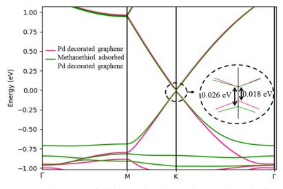
Figure 6. Band structure of Pd-decorated graphene and methanethiol adsorbed Pd-decorated graphene.
