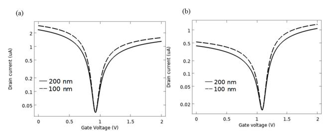
Figure 12. I-V characteristics as a function of dielectric layer thickness (a) AlP-GFET (b) Pd-GFET.
