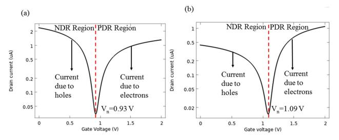
Figure 7. I-V characteristics show two distinct regions and the particular V<sub>n</sub> for (a) AlP-GFET, (b) Pd-GFET.
