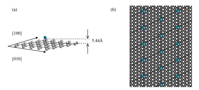
**Figure 3.** (**a**) The Pd-decorated graphene structure with C—Pd bond length; (**b**) extended surface of Pd decorated graphene considered for the energy band structure calculations.
