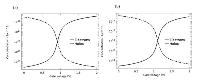
**Figure 8.** Carrier concentration in the graphene channel versus  $V_g$  for (**a**) AlP-GFET, (**b**) Pd-GFET. This confirms the occurrence of inversion of the device channel at  $V_n$ .
