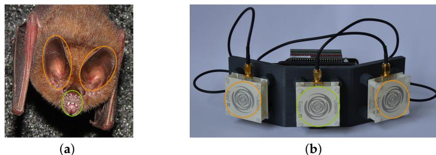
**Figure 1.** Comparison of the sensing mechanisms in biological echolocation and electronic echolocation. In both images, the emitter is marked green, and the receivers are marked orange. (a) The common big-eared bat (*Micronycteris microtis*). (b) A modified SensorLogic Ancho pulse-echo radar sensor.
