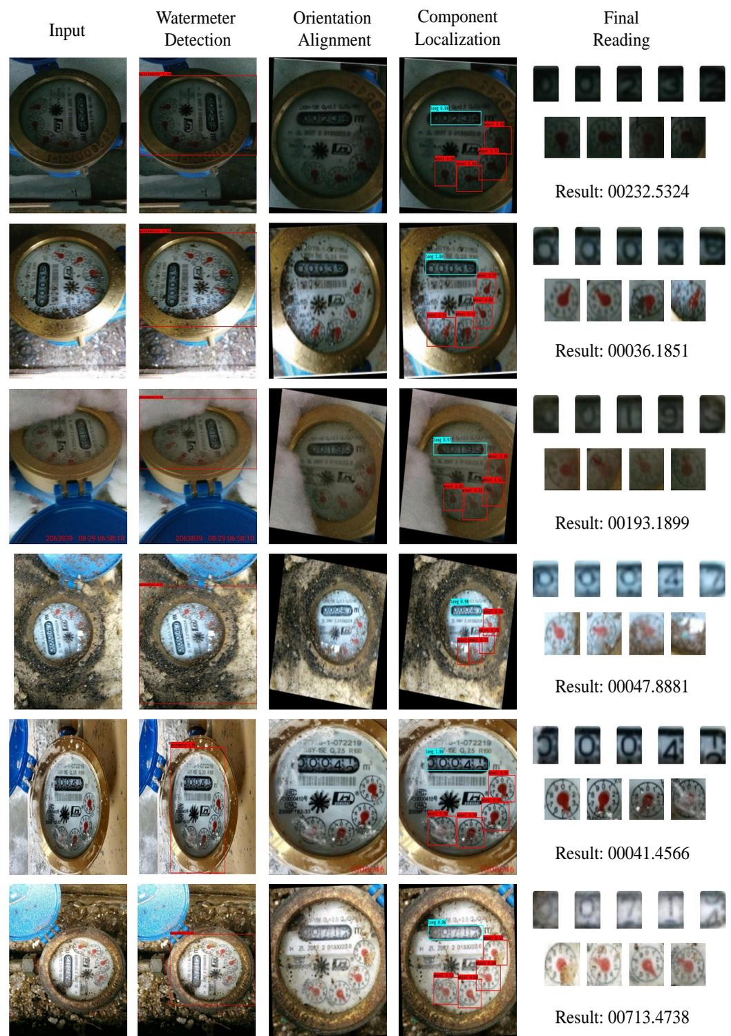
**Figure 13.** Performance test of the complete system: the first column is the input, the second to fourth columns are the intermediate results, and the last column is the final reading result.
