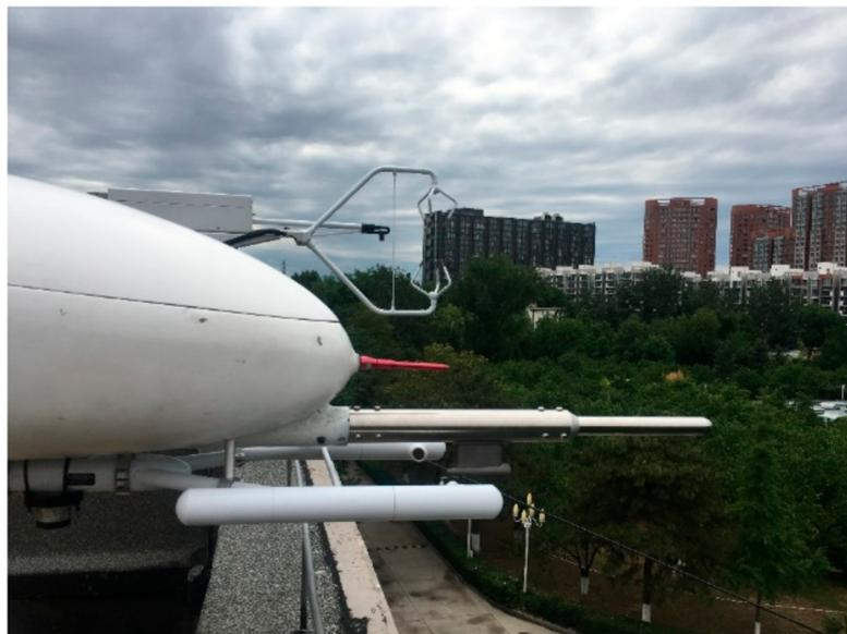
**Figure 3.** The ground-based comparison experiment between 1:00 and 6:00 p.m. on 31 May 2020 at the Chinese Research Academy of Environmental Sciences (CRAES) in Beijing ( $40^{\circ}2'27.51''$  N,  $116^{\circ}24'45.54''$  E) with a measurement height of 10.3 m above the ground level.
