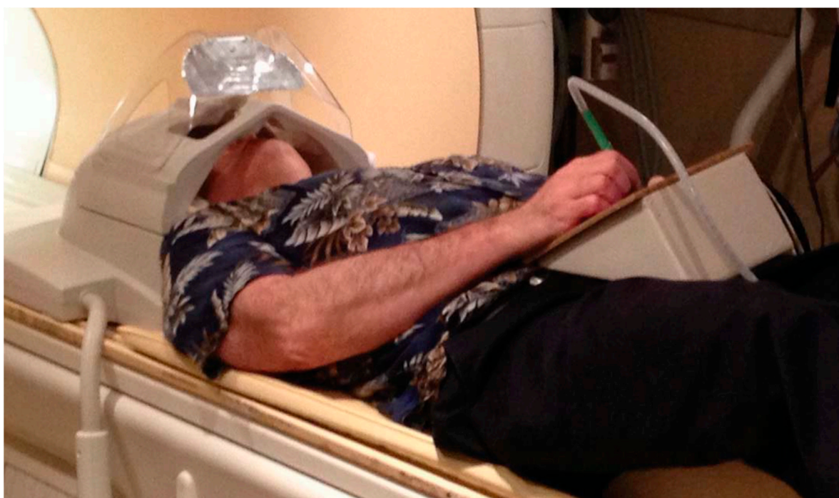
Figure 4. The fMRI-compatible Reitz tablet setup. The optical fibres are routed from the stylus tip to a light-tight box outside the magnet room. A mirror was mounted on the head coil to enable real-time visual feedback of task stimuli and response via video projection (not shown). Taken from [25]. Copyright © 2021 Reitz et al.
