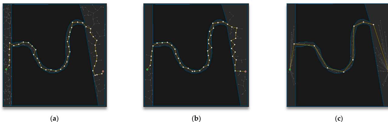
**Figure 11.** Experimental result of Map 1: (a) RRT; (b) RRT-Connect; (c) the proposed algorithm.
