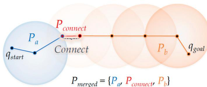
Figure 4. The ‘Connect’ method from the RRT-Connect algorithm.
