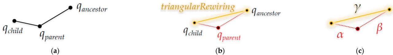
**Figure 5.** Abstract process of the ‘Triangular-Rewiring’ method: (a) Example tree; (b) After rewiring between  $q_{child}$  and  $q_{ancestor}$ ; (c) At this time,  $\alpha$  is the distance between  $q_{child}$  and  $q_{parent}$ ,  $\beta$  is the distance between  $q_{parent}$  and  $q_{ancestor}$ , and  $\gamma$  is the distance between  $q_{child}$  and  $q_{ancestor}$ .
