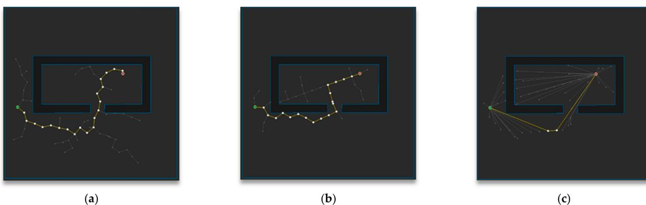
**Figure 12.** Experimental results of Map 2: (a) RRT; (b) RRT-Connect; (c) the proposed algorithm.
