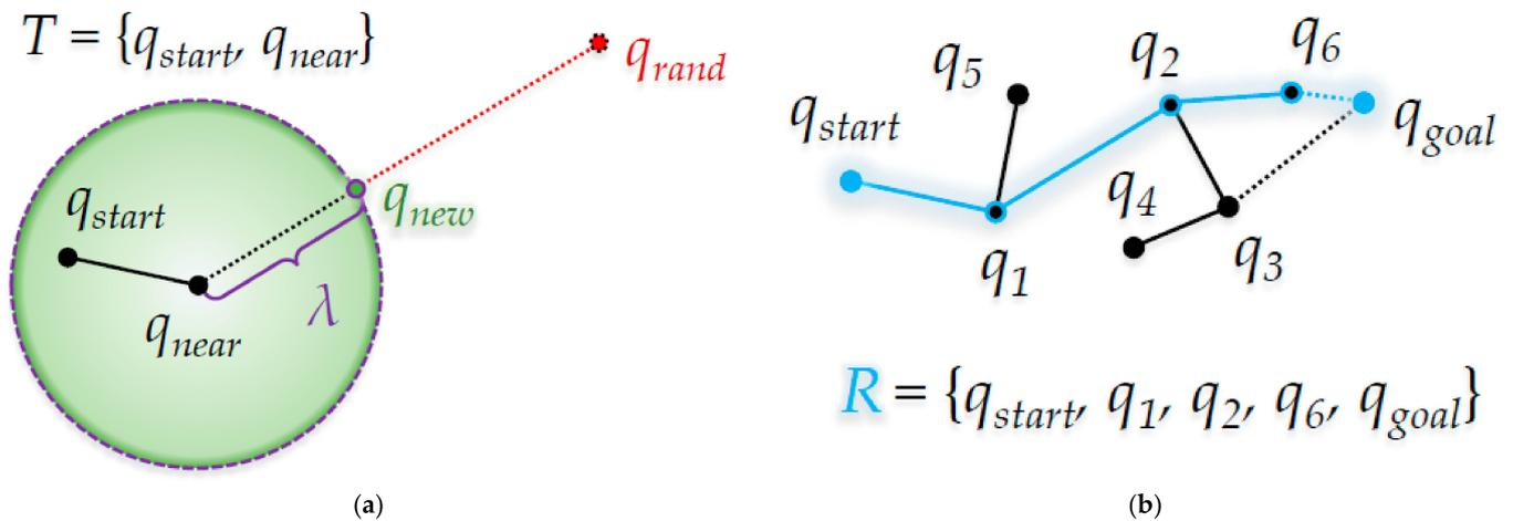
**Figure 2.** RRT algorithm: (a) Process when  $q_{new}$  is created; (b) After the random sampling has ended.
