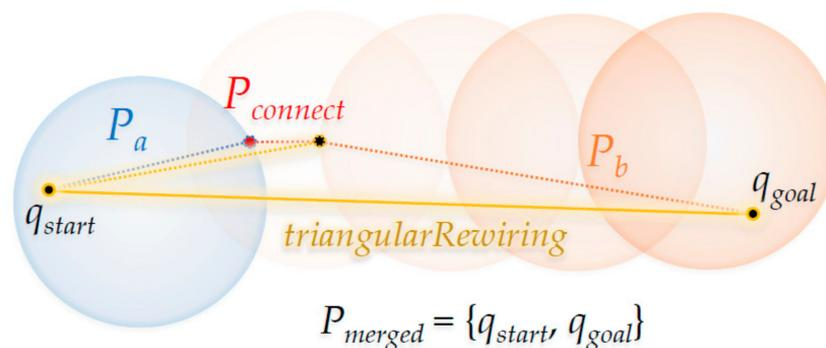
**Figure 8.** Proposed ‘Connect’ method for the RRT-Connect algorithm.
