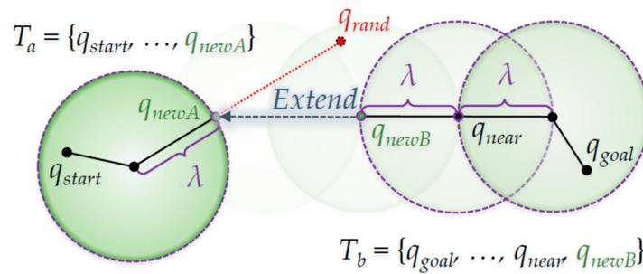
Figure 3. The ‘Extend’ method from RRT-Connect algorithm.
