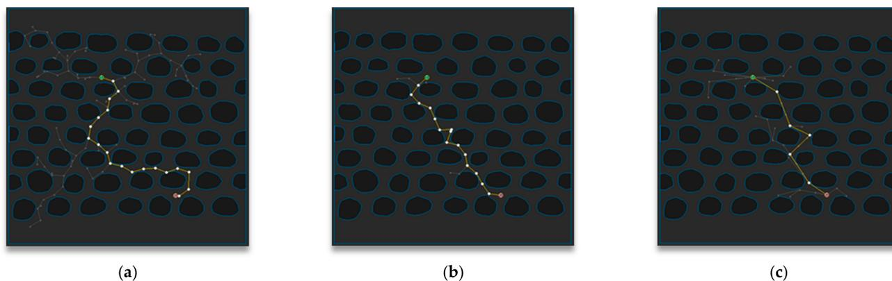
**Figure 15.** Experimental result of Map 5: (a) RRT; (b) RRT-Connect; (c) the proposed algorithm.
