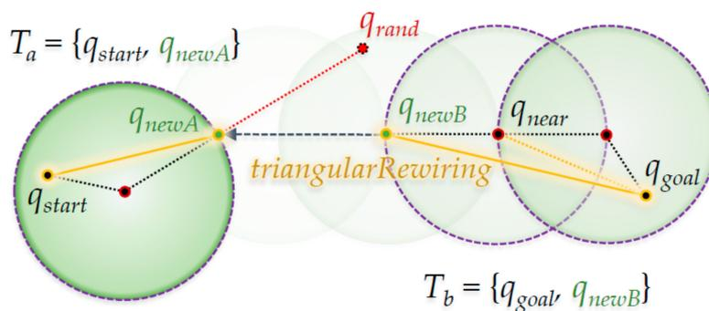
**Figure 7.** Proposed ‘Extend’ method for the RRT-Connect algorithm.
