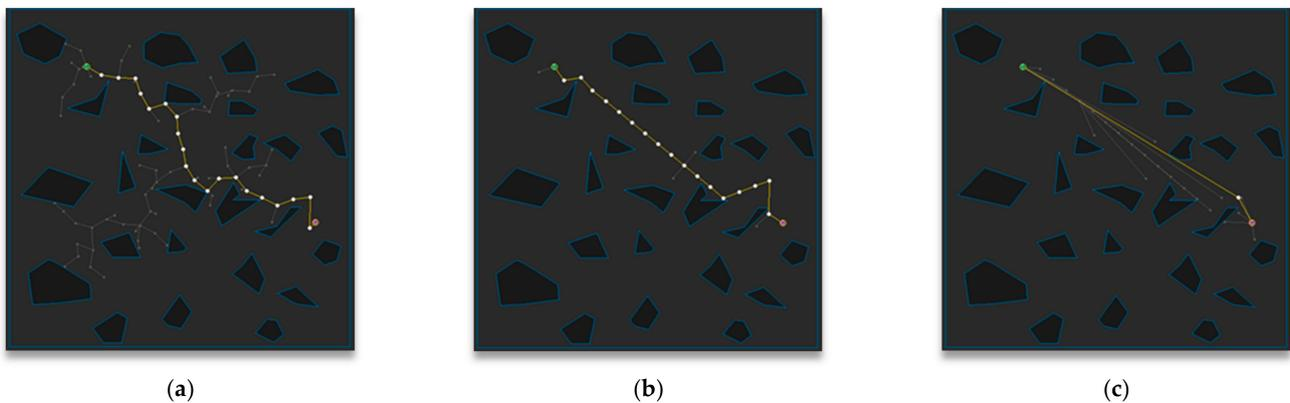
**Figure 14.** Experimental result of Map 4: (a) RRT; (b) RRT-Connect; (c) the proposed algorithm.
