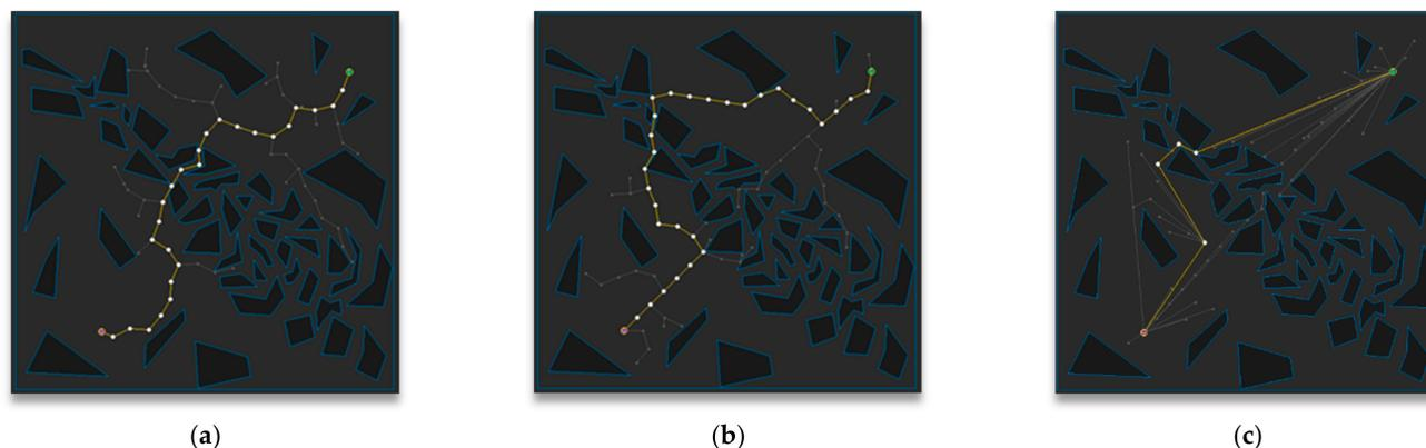
**Figure 16.** Experimental result of Map 6: (a) RRT; (b) RRT-Connect; (c) the proposed algorithm.
