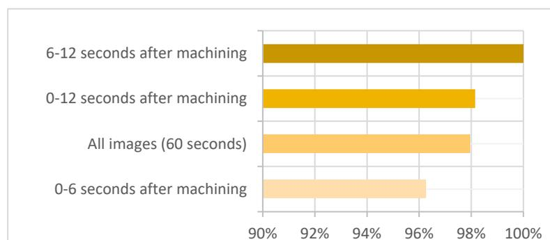
**Figure 6.** Accuracy for different classifications.
