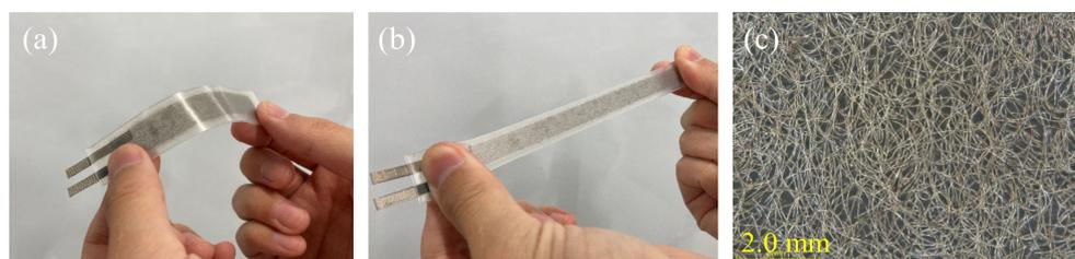
**Figure 3.** Appearances of the fabricated sensor ((a): non-stretched, (b): stretched) and a micrograph of the silver-plated fiber flocked in the conductive layer (c).
