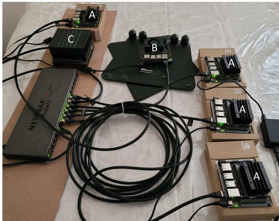
**Figure 5.** The prototype system: Devices labeled with “A” are Jetson Nanos, device “B” is the Jetson Xavier NX, and device “C” is the Jetson AGX Xavier.
