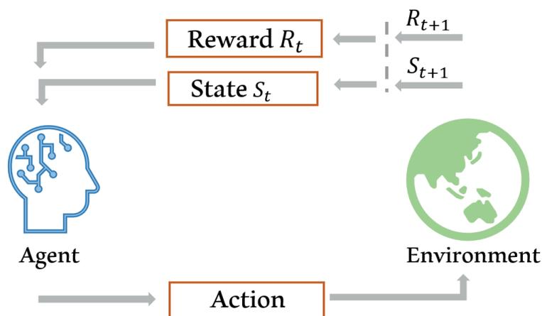
Figure 6. Reinforcement learning model diagram.
