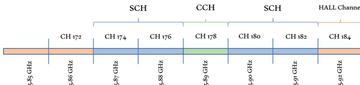
Figure 3. DSRC channel.
