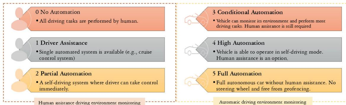
**Figure 2.** Autonomous vehicle levels by SAE.
