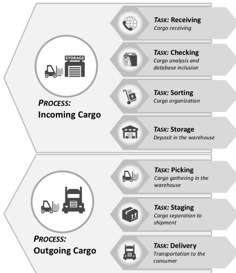
**Figure 4.** Description of processes, Incoming Cargo and Outgoing Cargo, and their tasks in warehouse logistics [42] (© 2020 IEEE).
