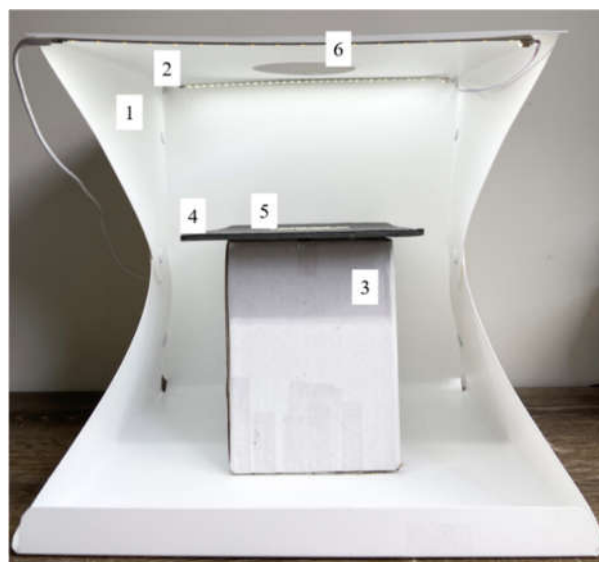
Figure 1. Experimental setup for image acquisition consisting of (1) a lightbox; (2) 70 pieces of two LED light strips; (3) a platform; (4) cardboard to place the grain for image acquisition; (5) rice samples; (6) top opening of the lightbox used to acquire the images using a smartphone. LED = light-emitting diode.
