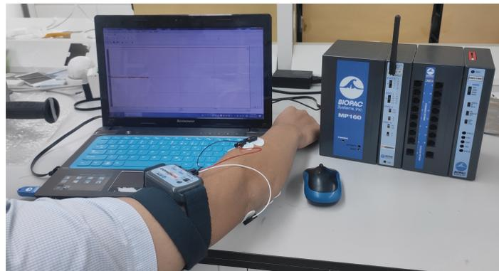
**Figure 2.** sEMG signal acquisition platform.
