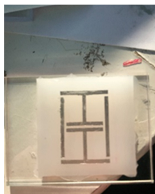
Figure 6. Finished Ecoflex tag with conductive ink.
