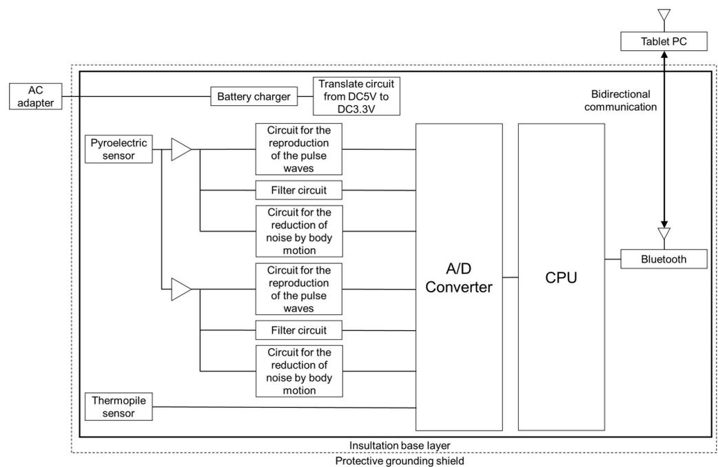
**Figure 3.** The system block diagram of the steering-type measurement system developed by Arakawa et al.
