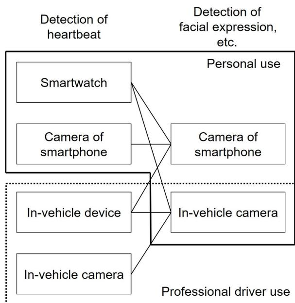
**Figure 7.** Segregation of the device for detection of heartbeat and expression. The lines connected from each block of “Detection of heartbeat” to each block of “Detection of facial expression, etc.” show the possible combination for adapting in-vehicle use.
