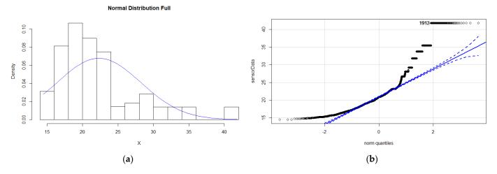
**Figure 3.** This figure shows the graphical analysis of data distribution for the Figure 2 temperature dataset with a bias fault injected: (a) Histogram of the temperature dataset; (b) *Q*-*Q* plot of the same temperature dataset, showing the deviation from a normal distribution (skewed right).
