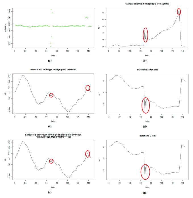
**Figure 4.** This shows an example of atmospheric pressure outlier detection with homogeneity tests: (**a**) Full dataset with atmospheric pressure metrics, with outliers; (**b**) Graph of the statistic calculated with SNHT; (**c**) Graph of the statistic calculated with Pettitt; (**d**) Graph of the statistic calculated with Buishand range test; (**e**) Graph of the statistic calculated with Lanzante's test; (**f**) Graph of the statistic calculated with Buishand U test.
