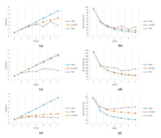
Figure 10. Graphs showing the performance of the parallel version of the scripts. (a) Speedup for the variation script.(b) Execution time for the variation script. (c) Speedup for the outlier script. (d) Execution time for the outlier script.(e) Speedup for the correlation script. (f) Execution time for the correlation script.
