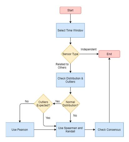
Figure 8. Process for analyzing correlation with other sensors.
