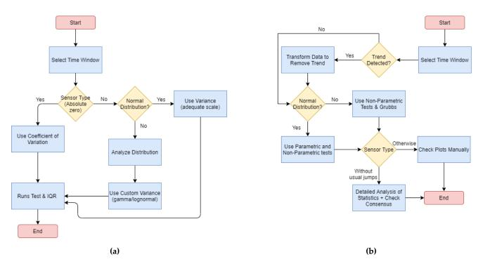
**Figure 7.** Processes for analyzing data from sensors: (a) Process to analyze variation of data; (b) Process for analyzing the presence of outliers in the data.
