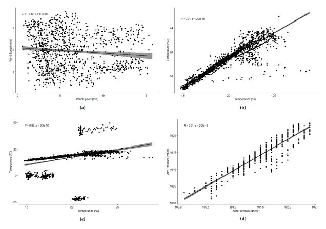
**Figure 5.** This figure shows the correlation diagram for different types of sensors and datasets: (**a**) Spearman correlation for wind speed (1 week); (**b**) Spearman correlation for temperature without errors (1 week); (**c**) Spearman correlation for temperature with drift errors (1 week); (**d**) Spearman correlation for atmospheric pressure (1 month), with different measurement units.
