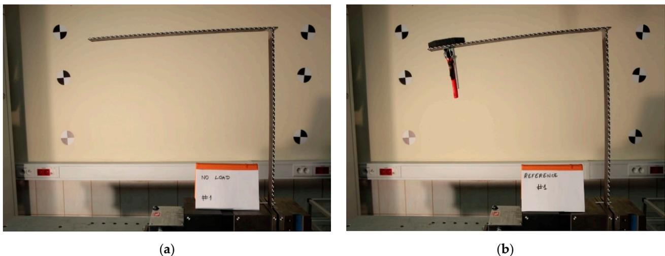
**Figure 3.** Images of the structure captured in the tests: unloaded state (a) and loaded state (b).
