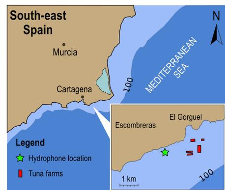
**Figure 7.** Cartagena region, showing the tuna farm and the UNDEX sites (red squares) as well as the hydrophone location (green star). The distance from the UNDEX to the hydrophone was approximately 1.2 km.
