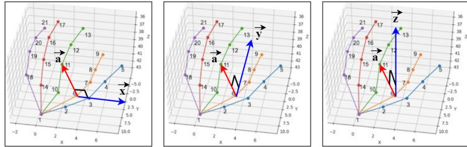
**Figure 5.** Calculation of angle-based features. Here,  $\vec{a}$  is a vector created by 6th and 11th joints. After that, the angles between  $\vec{a}$  and X-axis (**left**), Y-axis (**middle**), and Z-axis (**right**) have been calculated.
