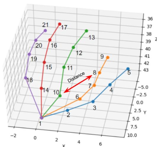
**Figure 4.** An example of distance-based features. Here, the distance between 8th and 10th joint points is being measured.
