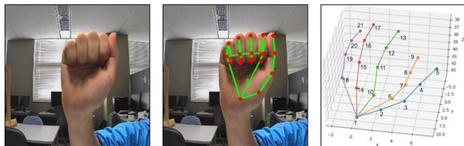
**Figure 3.** Using media-pipe API to obtain 21 joint points. The image in the left is an input image, the image in the middle is presenting the estimated joints and the image in the right is showing the joint order.
