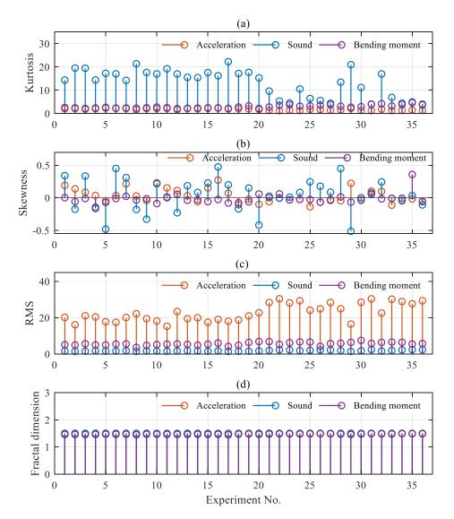
Figure 5. Distribution of features for different process parameters. (a) kurtosis; (b) skewness; (c) RMS; (d) fractal dimension.
