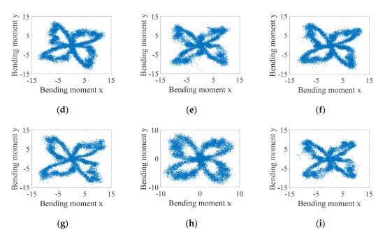
**Figure 9.** Polar plot of cutting bending moment for stable milling condition. (**a**) No. 1 experiment; (**b**) No. 2 experiment; (**c**) No. 3 experiment; (**d**) No. 4 experiment; (**e**) No. 5 experiment; (**f**) No. 6 experiment; (**g**) No. 7 experiment; (**h**) No. 8 experiment; (**i**) No. 9 experiment.
