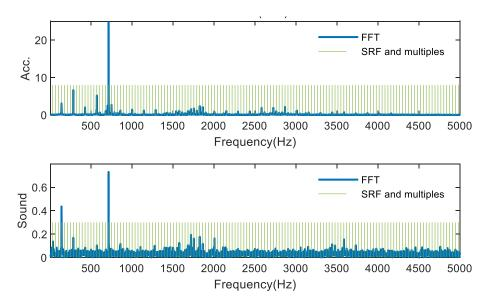
Figure 7. FFT for stable milling state experiments.
