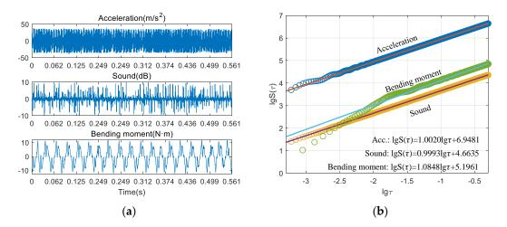
**Figure 3.** Calculation of the fractal dimension of the stable milling condition. (**a**) aquired signals; (**b**) process of calculating fractal dimension.
