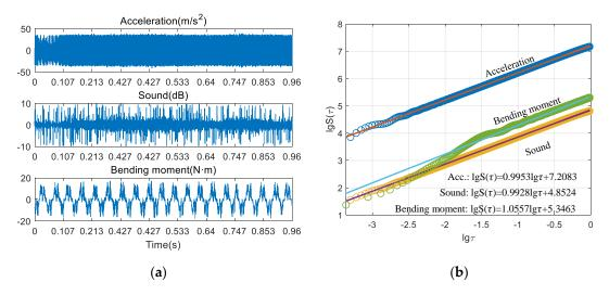
**Figure 4.** Calculation of the fractal dimension of the chatter condition. (**a**) aquired signals; (**b**) process of calculating fractal dimension.
