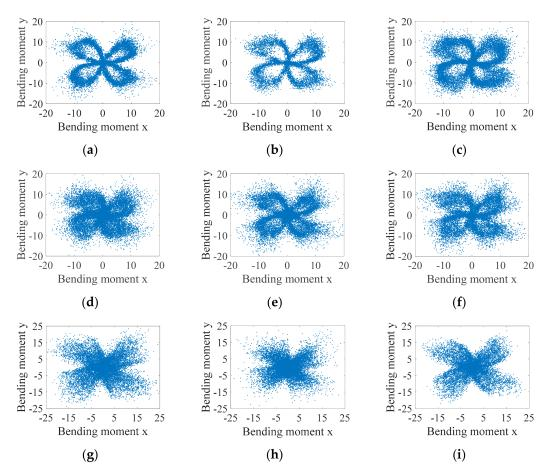
**Figure 10.** Polar plot of cutting bending moment for chatter milling condition. (**a**) No. 10 experiment; (**b**) No. 11 experiment; (**c**) No. 12 experiment; (**d**) No. 13 experiment; (**e**) No. 14 experiment; (**f**) No. 15 experiment; (**g**) No. 16 experiment; (**h**) No. 17 experiment; (**i**) No. 18 experiment.
