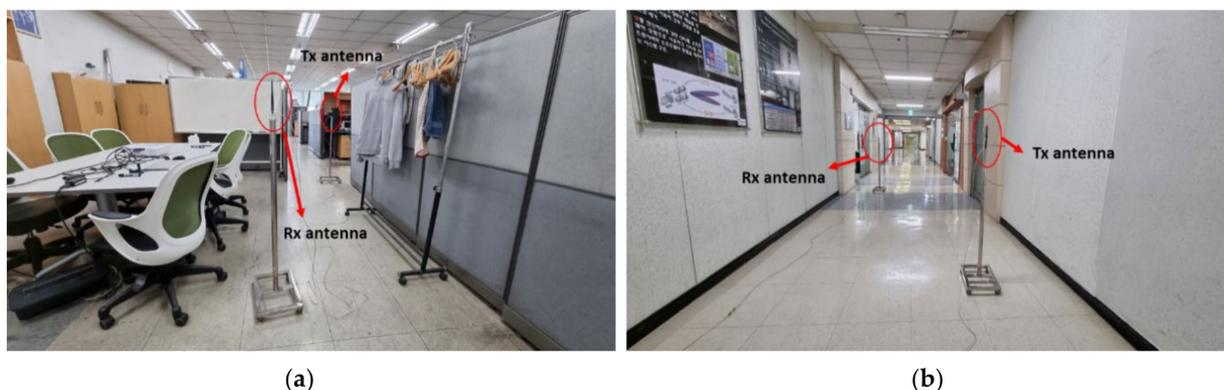
**Figure 19.** Experimental environments (a) Narrow laboratory with various furniture. (b) Relatively wide corridor.
