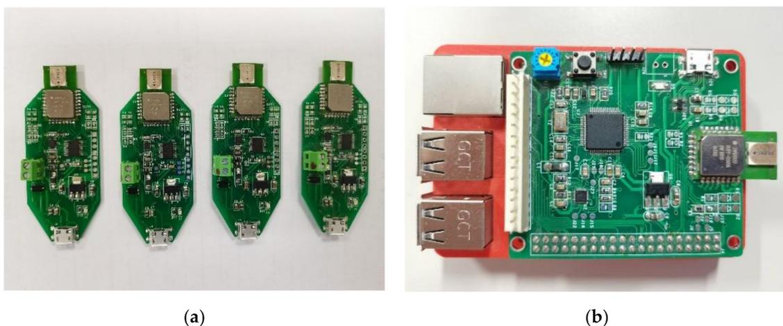
**Figure 1.** The UWB sensors used in this paper. (a) anchors; (b) mobile node.
