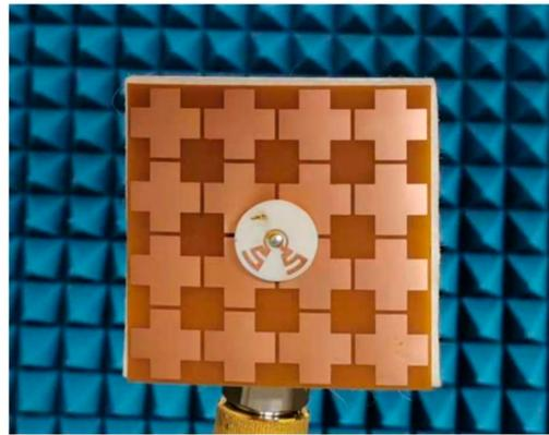
Figure 8. The prototype of the proposed antenna sensor.
