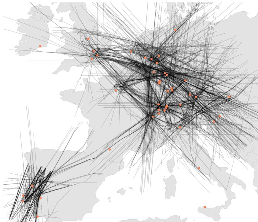
**Figure 5.** Verified aircraft and sensor positions in LocaRDS. The subset was created by using the provided indicator that measured the reliability of location and timing information from a specific aircraft and sensor.
