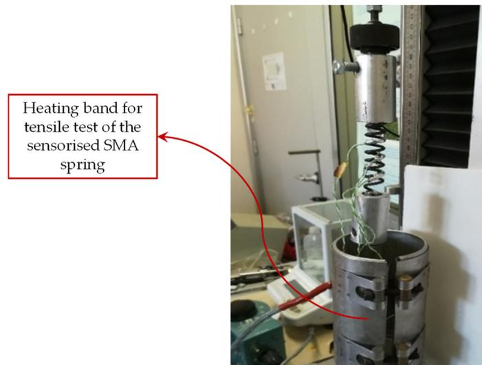
**Figure 13.** Electric resistance band used as a heating system.
