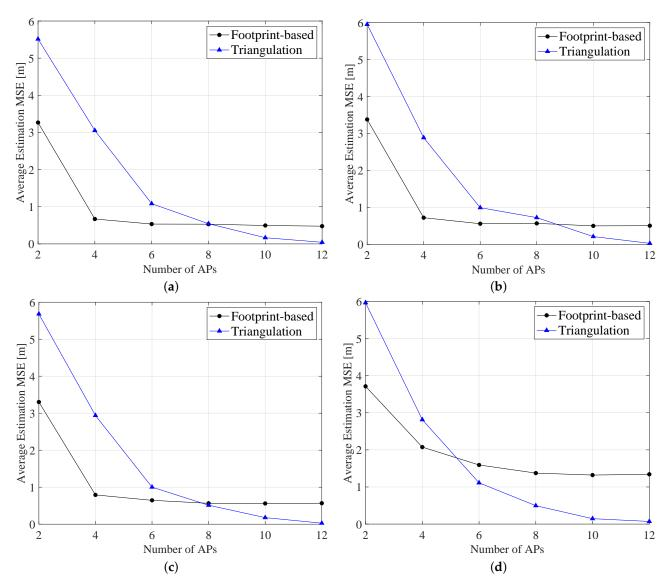
**Figure 7.** Average MSE comparison of fingerprint to triangulation approaches versus the number of APs and for different water types, i.e., (a) pure, (b) clear, (c) coastal and (d) harbor water. We assume a beam angle of  $60^{\circ}$ .
