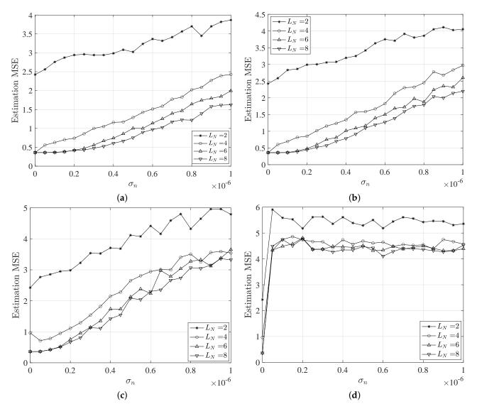
**Figure 3.** MSE of the position estimation behavior versus the noise standard deviation for different network configurations and water types, i.e., (a) pure, (b) clear, (c) coastal and (d) harbor water. We assume a beam angle of  $50^{\circ}$ .
