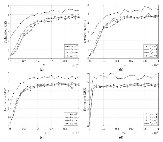
**Figure 4.** MSE of the position estimation behavior versus the noise standard deviation for different network configurations and water types, i.e., (a) pure, (b) clear, (c) coastal and (d) harbor water. We assume a beam angle of 80°.
