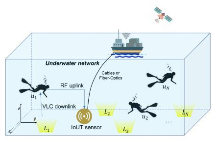
**Figure 1.** Schematic of a reference UVLC network, comprised of  $L_N=4$  LED transmitters and a centralized RF IoUT sensor node. Wearable battery-powered photodetectors are assumed to be placed on the diver's wetsuit.
