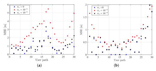
**Figure 5.** Comparison of MSE trends for different values of noise standard deviation computed for different user positions, for (a) variable and (b) fixed position along z-direction, i.e., z = 4 m.
