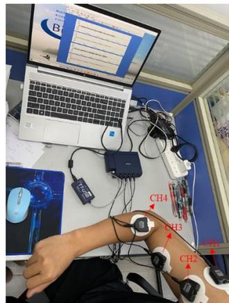
**Figure 3.** The position of patch electrodes and the sEMG acquisition equipment.
