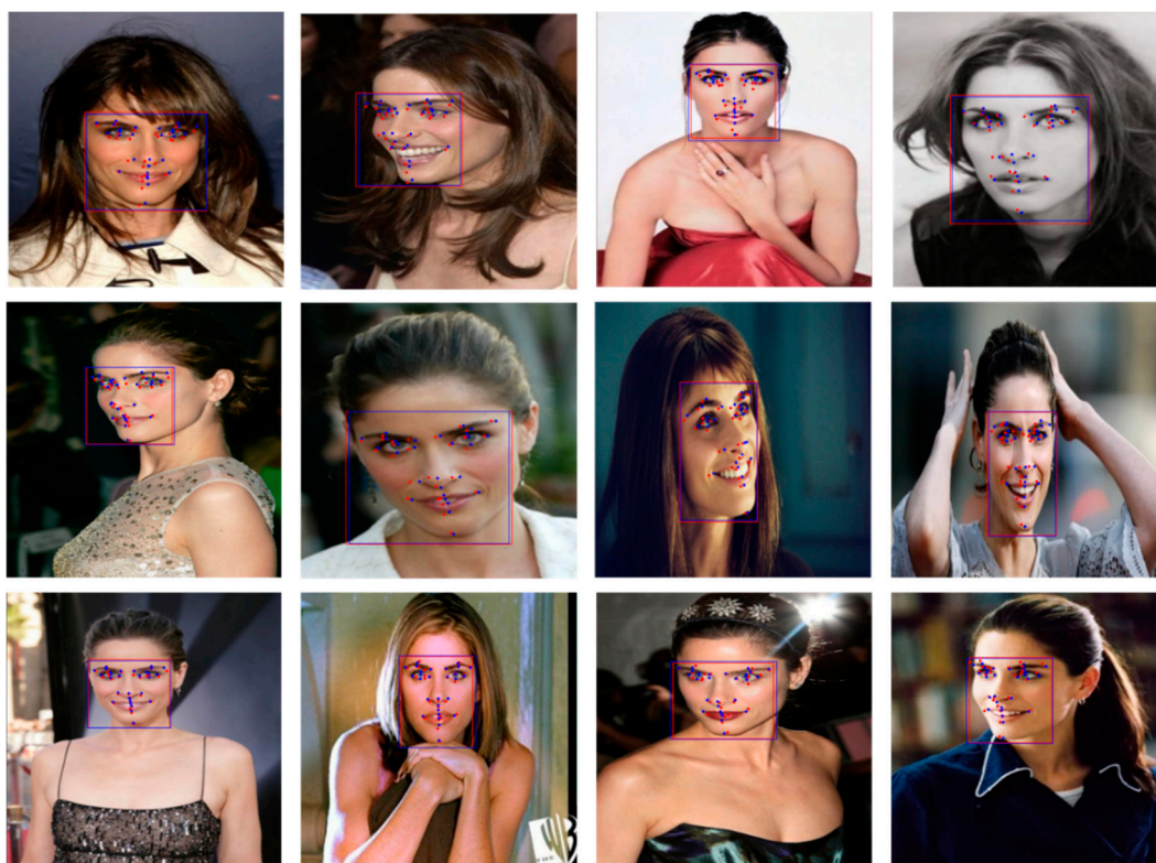
Figure 9. Test results of the proposed model of 29 landmarks. Blue dot: ground truth of face landmarks, Red dot: predicted face landmarks, Blue box: ground truth of face region, Red box: predicted face region.
