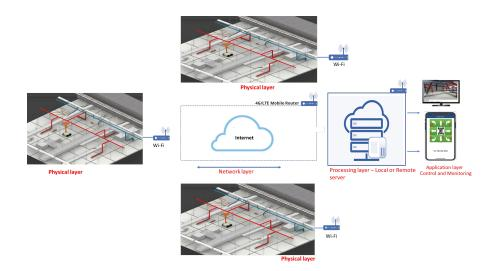
Figure 3. IoRT framework for rodent inspection in a false ceiling.
