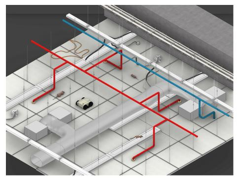
Figure 2. Overview of false ceiling inspection method using the Falcon robot.
