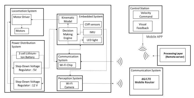
Figure 5. System architecture of Falcon.
