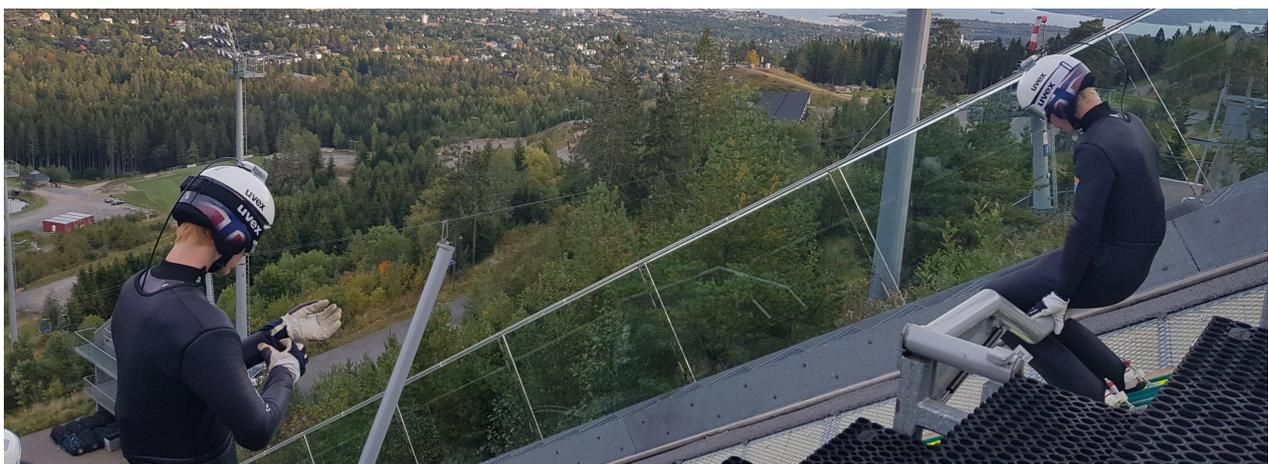
**Figure 2.** Ski jumpers with the dGNSS antennae mounted on their helmets and the receivers in backpacks that were carried under the ski jumping suit.
