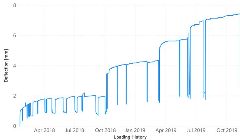
**Figure 4.** Evolution of midspan deflection along the loading history.
