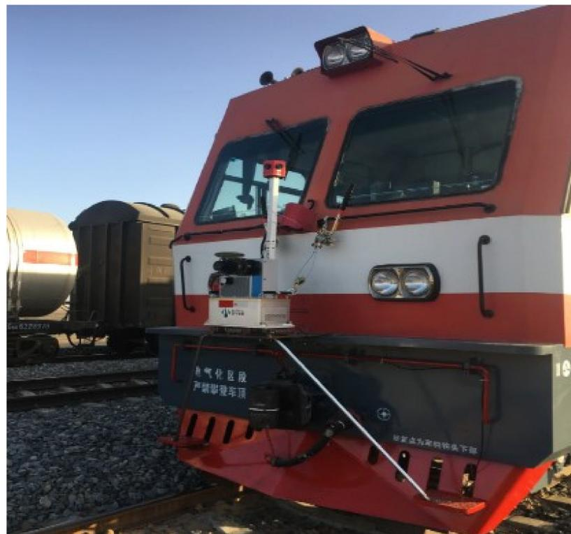
**Figure 4.** Vehicle-mounted LiDAR and its installation location.
