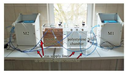
Figure 2. The measurement stand.
