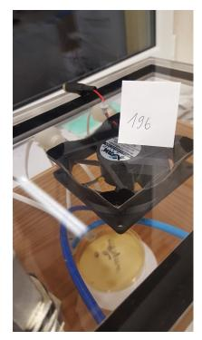
**Figure 5.** Measurement of a Petri dish with MYPGP media without visible colonies (class 23) in a wooden chamber.
