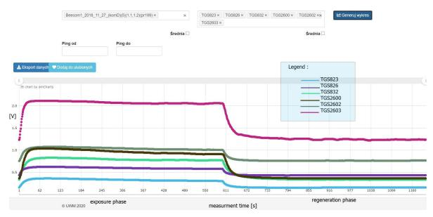
**Figure 6.** A sample graph illustrating the process of measurement. In this case, the measurement concerned a colony of *P. l. larvae* 6 days after culture in a wooden chamber.
