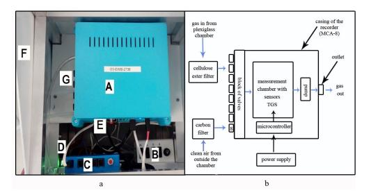
**Figure 1.** MCA-8 measurement device: (**a**) general view: A, multi-sensor recorder (MCA-8); B, power supply control panel; C, control panel for data transfer to the server; D, power cord; E, card reader; F, housing; and G, inlet channels; and (**b**) block diagram with marked construction elements and directional gas 80 flow.
