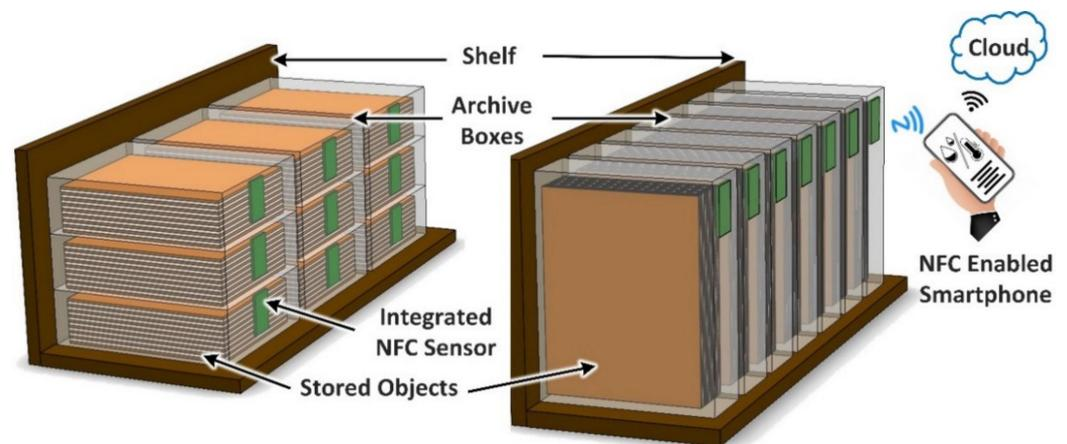
**Figure 1.** Illustration of the proposed solution for artifact storage monitoring using a novel battery-less temperature and humidity NFC sensor powered using a standard smartphone.
