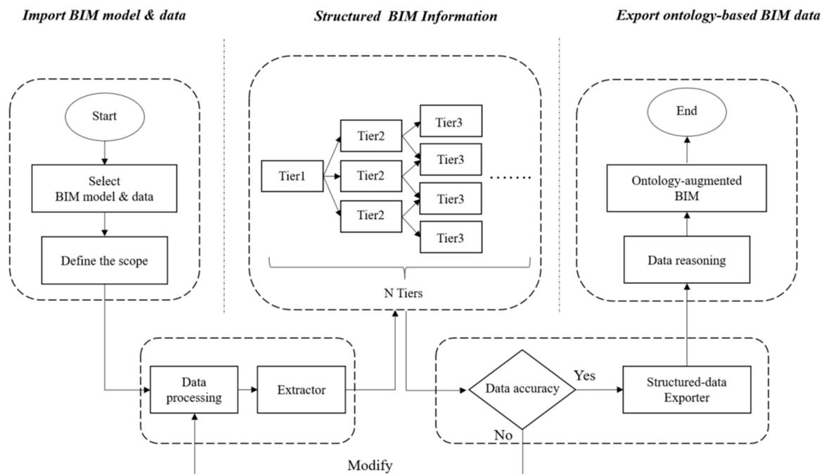
**Figure 2.** The process of structuring BIM data.
