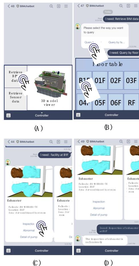
**Figure 13.** Example of the operation of the chatbot prototype using designed interface: (A) click Retrieve BIM data from the rich menu, (B) click Query by floor and select B1F from the imagemap, (C) find the designated facility and click Inspection, (D) the chatbot replies to the user with the inspection information.
