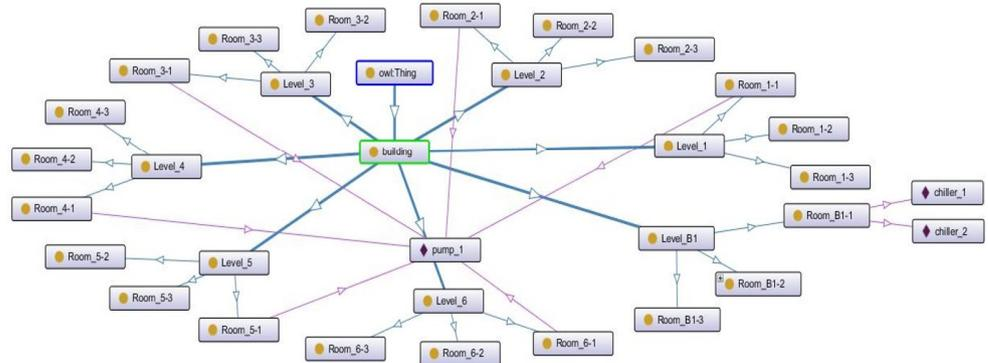
Figure 9. The ontology framework of the target building.
