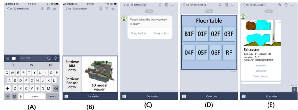
**Figure 12.** The main interface and menus of the chatbot: (A) the message input bar, (B) the rich menu, (C) confirm template, (D) imagemap message, and (E) carousel template.
