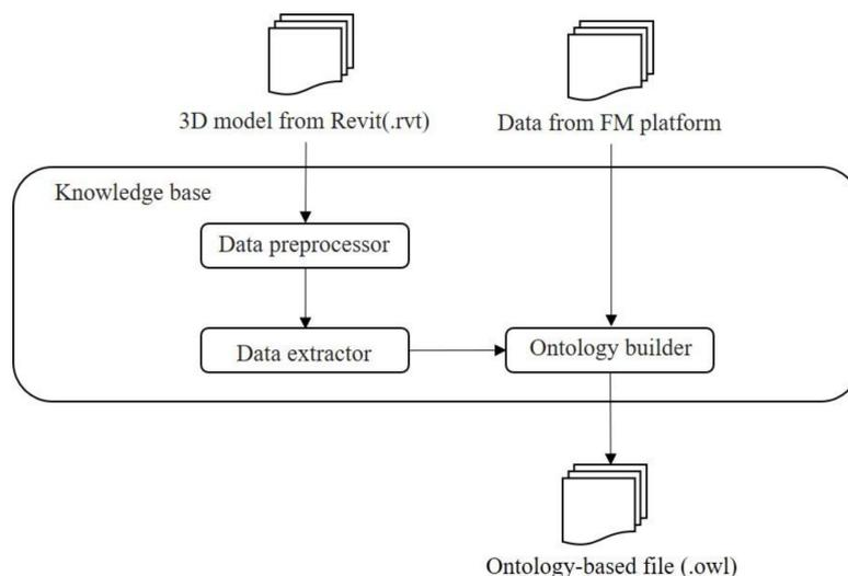
**Figure 8.** The workflow of knowledge base construction.
