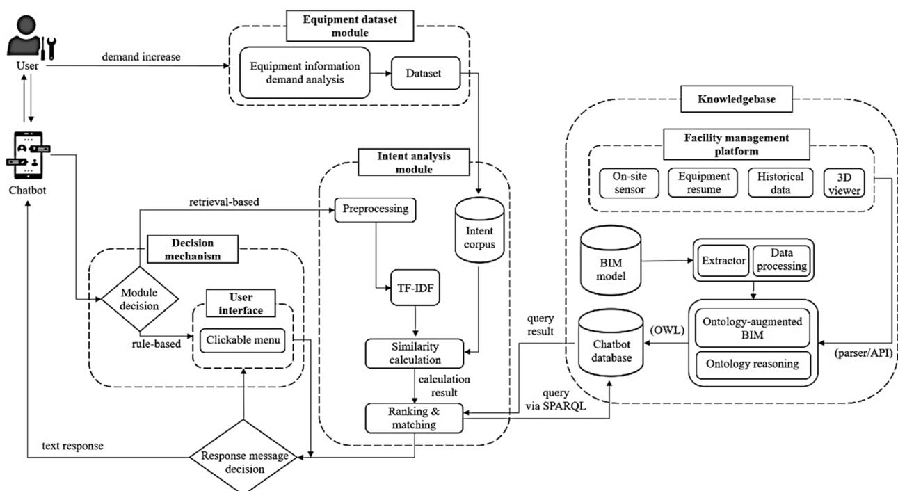
Figure 1. Conversation-based system architecture.
